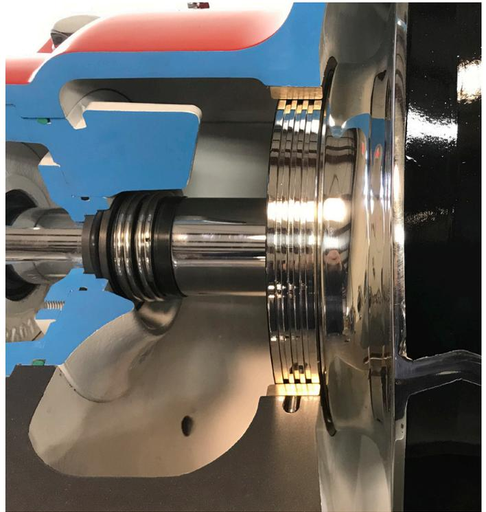
**In the above cutaway photograph of the mechanical seal chamber you can see the tapered bore which opens into the suction chamber of the pump. You can also see the axial rib above the seal that impacts the flow within the suction chamber.**
