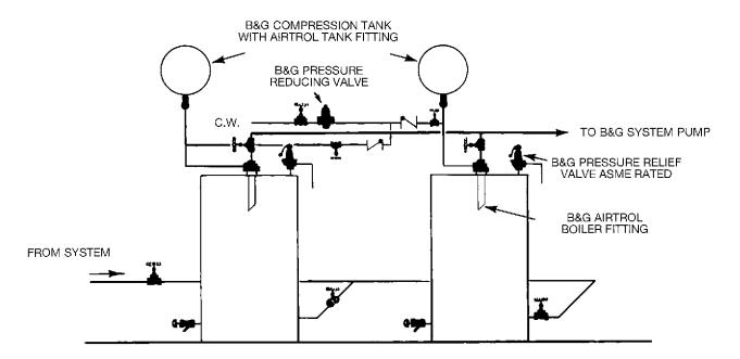
FIGURE 30 Multiple Boilers Incorrect Method
