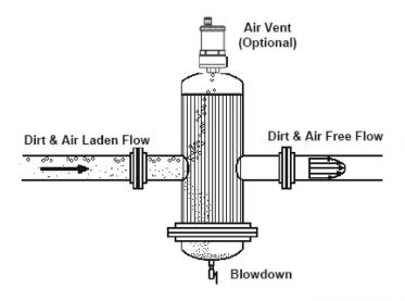
FIGURE 14 CRS Coalescing Removal Separator
