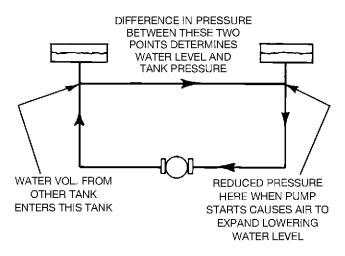
**NOTE:** When pump starts, point of no pressure change will be established somewhere between the two tanks depending upon change in water level of each.
