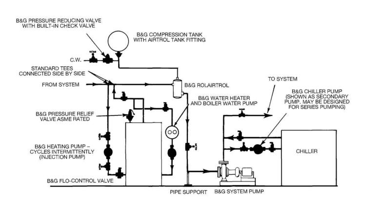
FIGURE 36 Air Control In Combination Heating/Cooling
