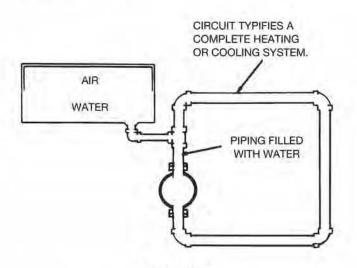
FIGURE 6 Basic Closed Hydronic Heating System
