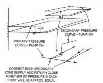
FIGURE 10 Primary/Secondary System Pressure Relationships
