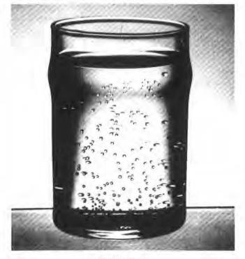
FIGURE 11 Air Bubbles Released From Fresh Tap Water With Pressure and Temperature Change
