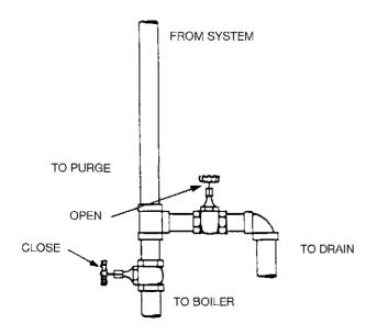
The purging hookup shown here is typical. Purging uses city water pressure to sweep the air in the system to a point where it is vented off. City water continues to flow until the discharge entering the drain is clear. Use care when city water pressures are high to ensure that the working pressures of all system components are not exceeded.
