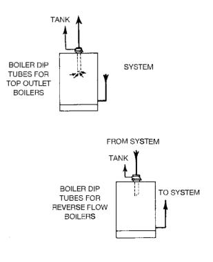
FIGURE 13 Boilers with Diptube Separators
