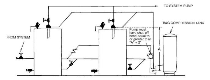
FIGURE 29 Multiple Boilers Alternate Method
