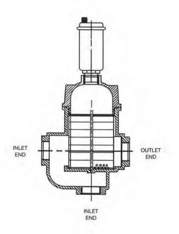
FIGURE 17 EAS Enhanced Air Separator
