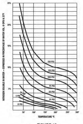
FIGURE 12 Solubility of Nitrogen in Water vs. Temperature and Pressure
