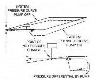
NOTE: Generally a poor location for system pump, illustration shows how pump pressure differential is subtracted from system pressures if pump differential is great enough to offset static head, cavitation, noise and pump damage may occur.
