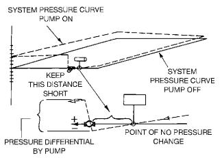
**NOTE:** Correct pump location adds pump pressure differential when operating away from point of no pressure change. Always keep distance short and pressure drop low between pump suction and compression tank connection.
