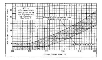
In the LTW range, as shown in the graph, adequate fill pressurization for a pump in any pressure that will prevent boiling plus a margin of safety, shown by the gray area. For example, a system with a 230° operating temperature should be filled to a minimum of 12 PSI where a system that operates at 240° must have a cold fill of 17 PSI at the pump.
