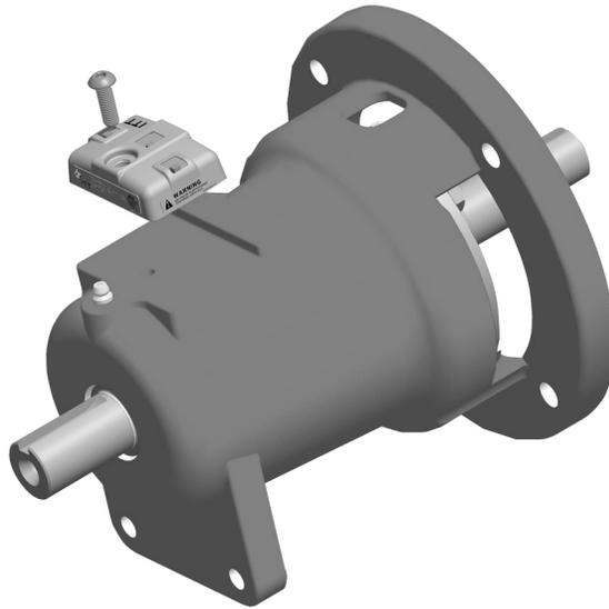
2. Tighten the hex-head screw with a 5/32 inch hex wrench to 6 ft-lbs (8 Nm).
