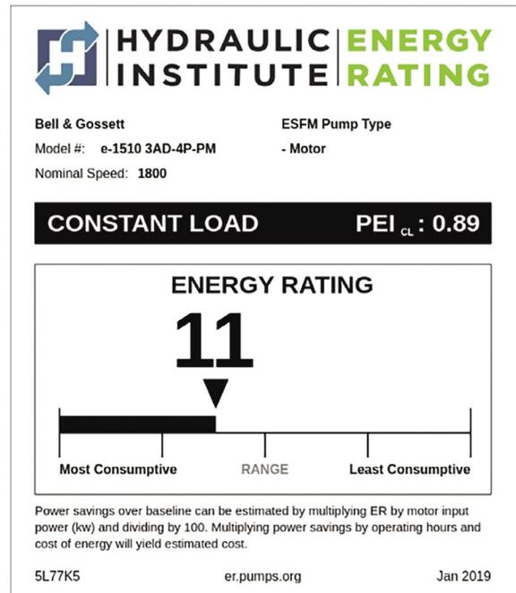
The bottom of the energy rating label provides information on how to estimate savings versus the baseline (PEI 1.0) end suction frame mounted pump. If Pump A's motor is 90 percent efficient and operates close to 5 hp, input power will be 5.55 hp, or 4.1 kW.
