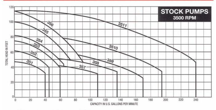
Add "S" to pump number when ordering single phase pumps. Add "T" to pump number when ordering three phase pumps.
