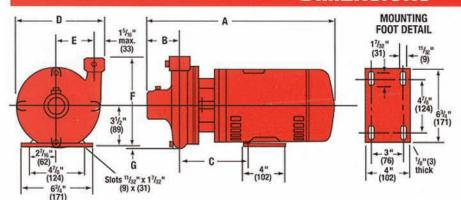
Bronze fitted Construction. Motors — Open Dripproof. Single Phase — Unit Number ending in "S", 115/230 Volt, 60 Cycle, 1 Phase. Three Phase — Unit Number ending in "T", 208-230/460, 60 Cycle, 3 Phase.
