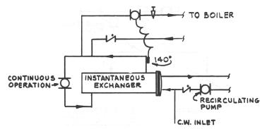
Figure 55 – INSTANTANEOUS DOMESTIC WATER CONTROLLED FROM SHELL SIDE
