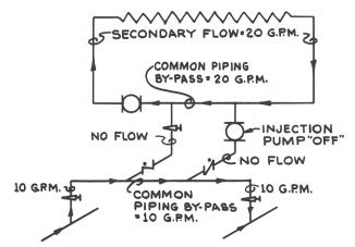
Figure 26 - SAME AS FIGURE 25, EXCEPT INJECTION PUMP OFF
