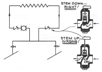
Figure 38 - FLO CONTROL STEM MUST BE DOWN
