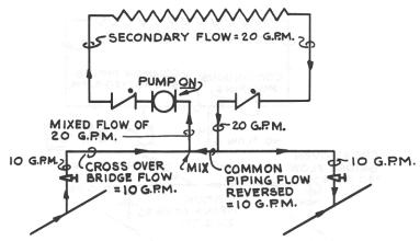
Figure 21 – STOP-START PUMP CONTROL PUMP ON, CROSS-OVER FLOW LESS THAN SECONDARY
