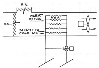
Figure 105 – CONVENTIONAL 3 WAY CONTROL TO AIR HANDLER
