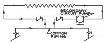
Figure 5 - WRONG-SECONDARY CIRCUIT PUMP DISCHARGES INTO COMMON PIPING
