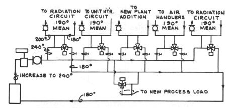
Figure 104 – INCREASED TEMP DROP BY P-S APPLICATION TO EXISTING DISTRIBUTION CIRCUIT PERMITS ADDITIONS WHILE USING EXISTING CIRCUIT.
