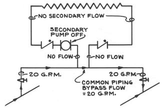
Figure 20 - SAME AS FIGURE 19 EXCEPT SECONDARY PUMP "OFF"
