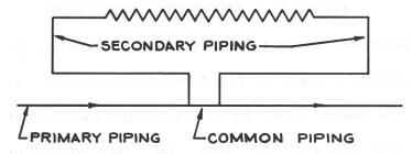
Figure 2 – BASIC PRIMARY-SECONDARY CONNECTION
