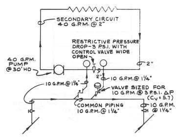
Figure 76 – TWO WAY - PRIMARY SECONDARY SIZING EXAMPLE
