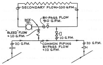
Figure 32 – SAME AS FIGURE 31 EXCEPT VALVE PARTIALLY CLOSED
