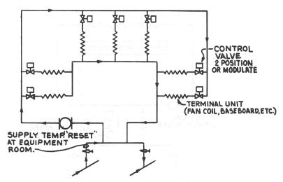
Figure 47 – SECONDARY ZONE PUMPING; ELIMINATION OF PRIMARY HEAD EFFECT ON TERMINAL UNIT CONTROL
