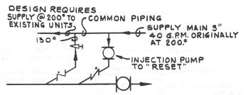
Figure 100 - EXAMPLE 3 FLOW DIAGRAM; HEAT SOURCE TAP INTO SUPPLY MAIN
