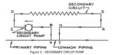
The secondary circuit pump is sized to provide design flow rate through the secondary circuit with reference to secondary circuit pressure drop only. In the sketch shown in Figure 3 this includes pressure drops; A-B, B-C, C-D, D-E, E-G and H-I. Since the common piping pressure drop (A-I) is slight, it will have no effect on secondary circuit pumping requirements and the secondary circuit can be considered separately and in hydraulic isolation from the primary circuitry.
