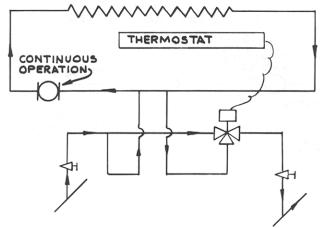
Figure 66 – AIR HANDLER-FREEZE PROTECTION PLUS AIR TEMP. CONTROL
