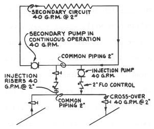
Figure 50 – INJECTION SIZING; CROSS-OVER FLOW EQUAL TO SECONDARY FLOW
