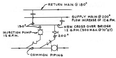
Figure 102 – CROSS OVER BRIDGE APPLICATION TO EXAMPLE 2
