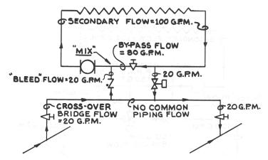
Figure 31 – TWO WAY MODULATING VALVE CONTROL; APPLY ONLY WHEN CROSS OVER FLOW IS LESS THAN 30% IF SECONDARY; VALVE WIDE OPEN
