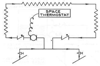
Figure 41 – CONTROL OF BASEBOARD SECONDARY CONTROL
