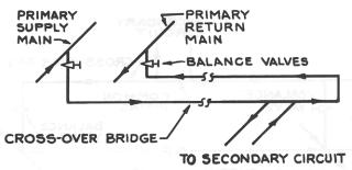
Figure 9 - CROSS-OVER BRIDGE PIPING LENGTH
