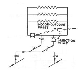
Figure 52 – RESET CONTROL SECONDARY ZONE
