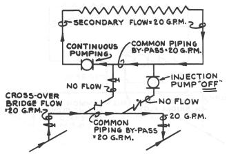
Figure 24 – SAME AS FIGURE 23 EXCEPT INJECTION PUMP OFF
