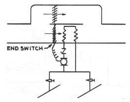
Figure 45 – FACE AND BYPASS DAMPER CONTROL TO ELIMINATE "HEAT WIPE" & PERMIT DEEP TEMP. DROP DESIGN IF PRIMARY. SECONDARY PUMP "OFF" BY END SWITCH
