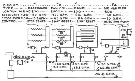
Figure 81 – POSSIBLE SECONDARY CIRCUIT CONTROL ARRANGEMENTS - DESIGN EXAMPLE
