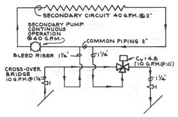
Figure 63 - MODULATING THREE WAY; CROSS-OVER FLOW LESS THAN SECONDARY
