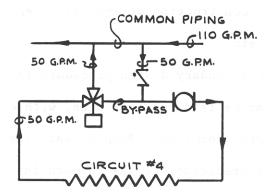
Figure 96 – THREE WAY BYPASS OR DIVERTING VALVE APPLICATION TO ONE PIPE PRIMARY MAIN
