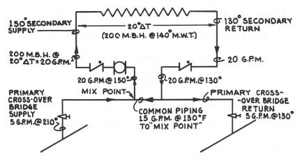
Figure 35 - DESIGN EXAMPLE FLOW RATES
