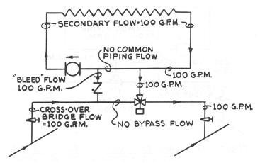
Figure 27 – MODULATING 3 WAY VALVE CONTROL; CROSS-OVER BRIDGE FLOW = SECONDARY; VALVE WIDE OPEN – BYPASS CLOSED
