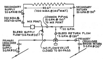
Figure 36 - DESIGN EXAMPLE FLOW RATES - 3 WAY VALVE APPLICATION
