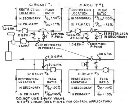
Figure 94 - TWO WAY MODULATING CONTROL EXAMPLE FOR ONE PIPE PRIMARY
