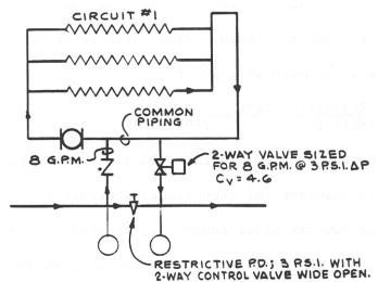
Figure 95 – TWO WAY MODULATING AND RESTRICTIVE P.D. RELATIONSHIP
