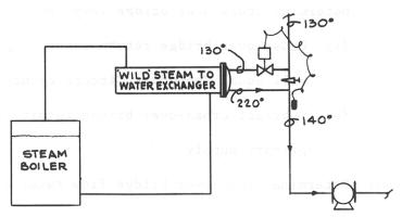
Figure 79 – TWO WAY MODULATING "RESET" CONTROL APPLIED TO HEATING SIDE OF HEAT-COOL SYSTEM WITH WILD STEAM TO WATER EXCHANGER
