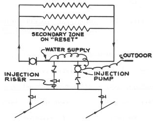
Figure 48 – INJECTION PUMP APPLICATION TO "RESET" SECONDARY ZONE
