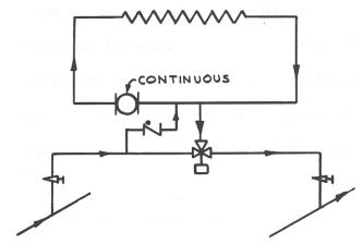
Figure 61 - MIXING VALVE IN CROSS-OVER PIPING - OVERHEAD
