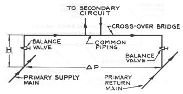
Figure 7 – CROSS-OVER BRIDGE OVERHEAD
