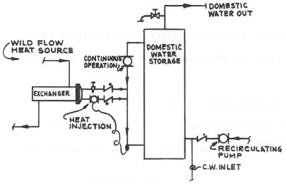
Figure 54 – CIRCULATED DOMESTIC WATER STORAGE TANK
