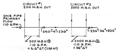
Figure 86 – TEMPERATURE DROP SEQUENCE ONE PIPE PRIMARY MAIN
