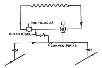
Figure 59 – BYPASS OR DIVERTING VALVE IN SECONDARY
