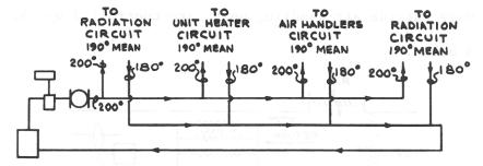
Figure 103 – EXISTING DISTRIBUTION PIPING CONVENTIONAL 20° ΔT DESIGN
