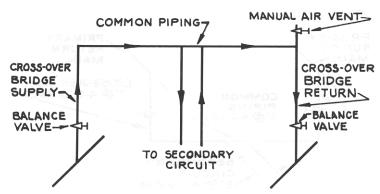
Figure 8 - CROSS-OVER BRIDGE WITH MANUAL VENT
