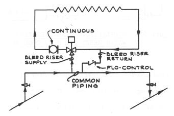
Figure 58 – MIXING VALVE APPLICATION IN SECONDARY CIRCUIT
