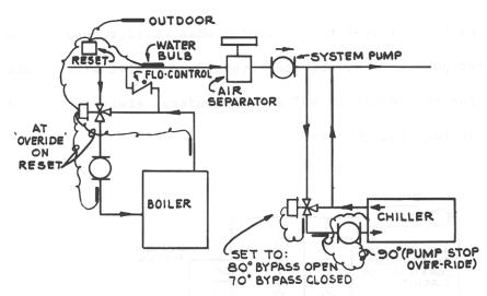
Figure 69 – SIMPLE CHANGE-OVER, RESET OF HOT WATER, BOILER SHOCK PROTECTION, CHILLER USED TO COOL DOWN "HOT" SYSTEM ON CHANGE-OVER CHILLER STEP CONTROL NOT EFFECTED BY CHANGES IN SYSTEM FLOW RATE.
