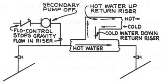
Figure 39 - GRAVITY FLOW - SINGLE PIPE
