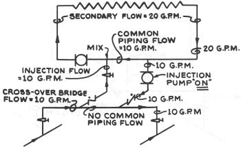
Figure 25 – INJECTION PUMP CONTROL CROSS-OVER BRIDGE FLOW LESS THAN SECONDARY INJECTION PUMP ON
