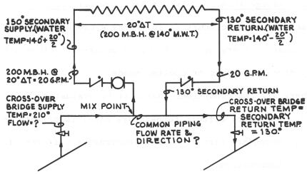
Figure 34 – DESIGN EXAMPLE; DETERMINATION OF CROSS-OVER BRIDGE FLOW RATES
