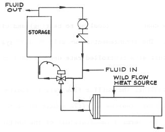
Figure 68 – INDUSTRIAL FLUID TEMP CONTROL
