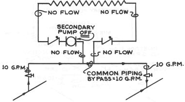
Figure 22 - SAME AS FIGURE 21 EXCEPT SECONDARY PUMP "OFF"
