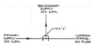
100 GPM (Primary In) = 100 GPM (Secondary out)
