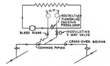
Figure 72 – TYPICAL APPLICATION; TWO WAY MODULATING CONTROL VALVE
