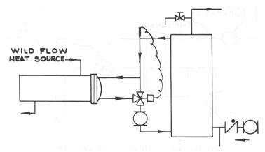
Figure 67 – CIRCULATED DOMESTIC WATER STORAGE TANK
