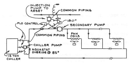
Figure 99 - EXAMPLE 2 FLOW DIAGRAM
