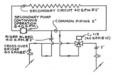
Figure 62 – MODULATING THREE WAY PIPE SIZING: CROSSOVER FLOW = SECONDARY
