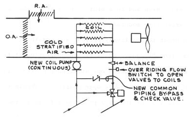
Figure 107 - COIL PUMP ADDITION FOR FREEZE PROTECTION 3 WAY VALVE (COMPARE WITH FIGURE 105)
