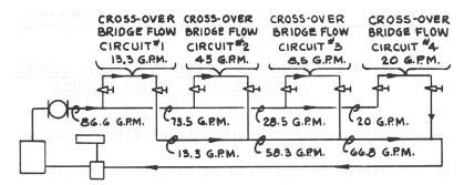
Figure 80 - REVERSE RETURN PRIMARY CIRCUIT FLOW RATES - DESIGN EXAMPLE
