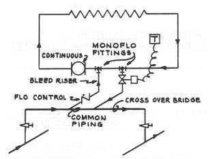
Figure 73 – TWO WAY VALVE; RESTRICTIVE FLOW CAUSING PRESSURE DROP BY MONOFLO FITTINGS
