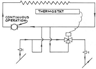
Figure 65 – SPACE TEMPERATURE CONTROL OF SECONDARY
