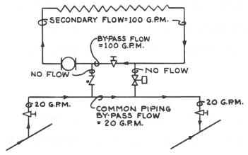
Figure 33 – SAME AS FIGURE 31 EXCEPT VALVE CLOSED
