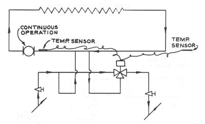
Figure 64 – INDOOR-OUTDOOR RESET OF SECONDARY
