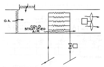
Figure 106 – CONVENTIONAL 2 WAY CONTROL TO AIR HANDLER
