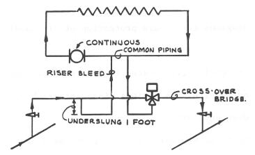
Figure 60 – MIXING VALVE IN CROSS-OVER PIPING – UNDERSLUNG RISERS
