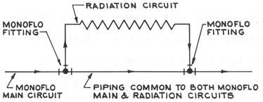
Figure 1 – TYPICAL MONOFLO CIRCUIT
