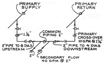
Figure 11 - CROSS-OVER BRIDGE PIPE SIZING: UNEQUAL P-S FLO:
