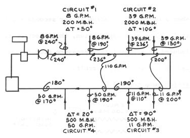
Figure 89 – TOTAL CIRCUIT; INJECTION RISER FLOW RATES
