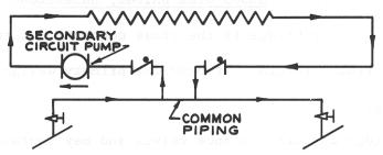
Figure 4 – RIGHT-SECONDARY CIRCUIT PUMP DISCHARGES INTO CIRCUIT
