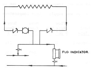
Figure 83 – FLO INDICATOR IN CROSS-OVER BRIDGE; DIRECT RETURN DESIGN
