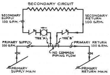
Figure 16 – COMPLETE CIRCUIT FLOW; PRIMARY FLOW = SECONDARY FLOW
