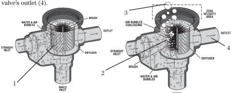
While the original EAS is cast iron with an external 3/4" high capacity air vent, the newer EASB-JR has a brass body and a built-in automatic air vent
