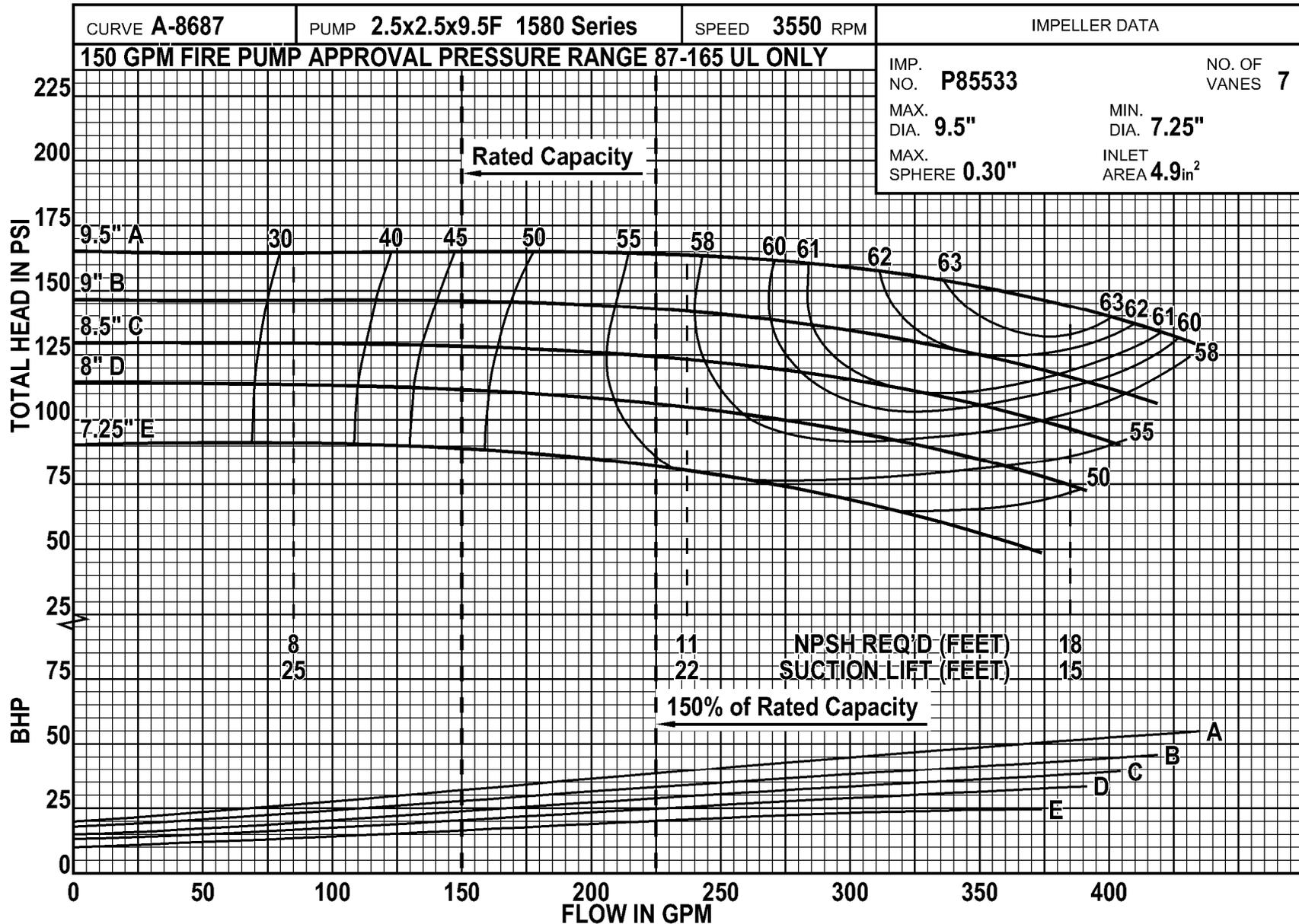
Curves show performance with clear water at 85°F. If specific gravity is other than 1.0, BHP must be corrected.
