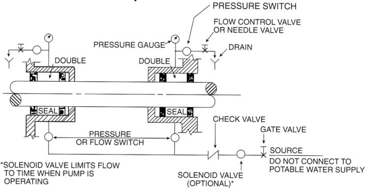
MINIMUM FLOW RATE = 0.5 GPM PER SEAL
