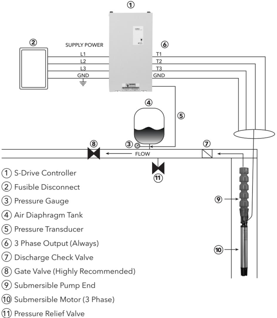
**NOTE:** for single phase input, connect L1 and L3, then set motor overload switches to 50% of controller rating or lower.
