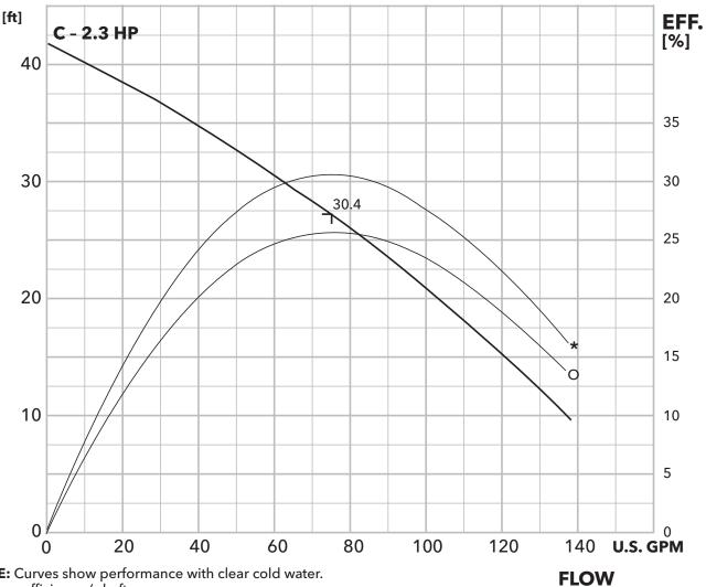
**NOTE:** Curves show performance with clear cold water. \*: Pump efficiency / shaft power
