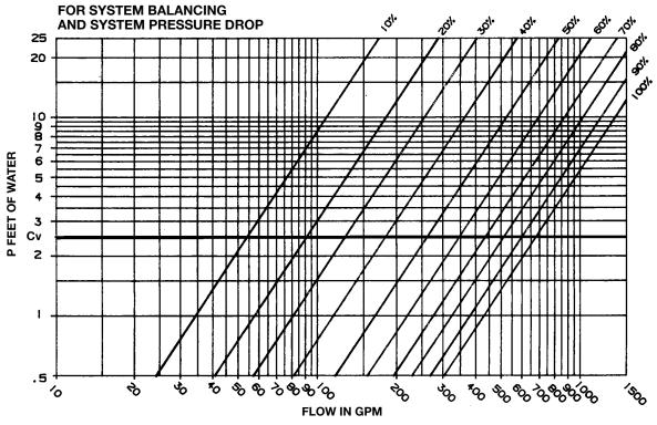
**MAXIMUM RECOMMENDED FLOW 1,140 GPM**
