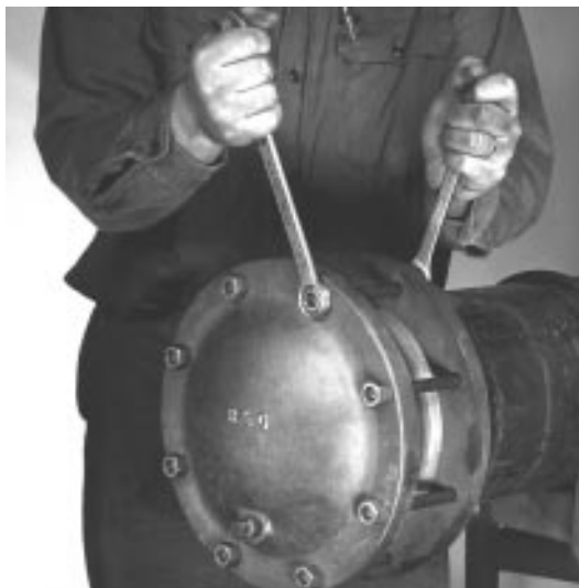
Illustration No. 2 – Removing rear head (completely remove front and rear heads).
