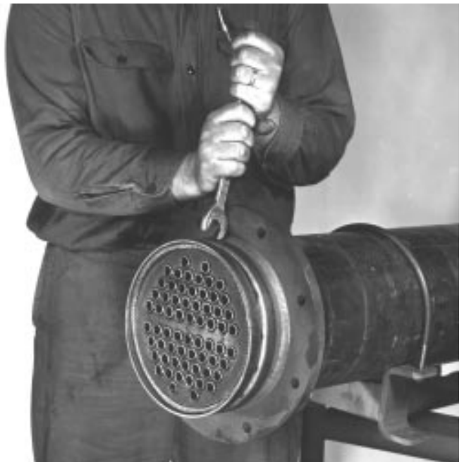
Illustration No. 4 – Prying off retainer rings.
