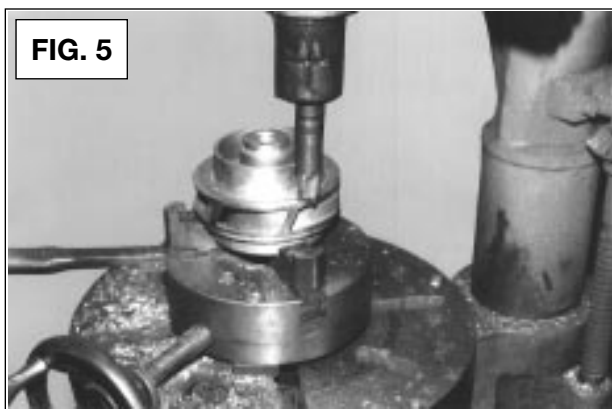
FIG. 5 STEP NO. 3 — Place impeller in chuck on drill table. Align flat mill cutting tool at center of imbalance point on the impeller wall. If the unbalanced condition is quite pronounced make the first cut about 1/64" deep and 2" to the left and right of the center point. This is done by moving the handle at-
